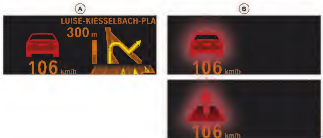
BMW 5 Series LCI Collision warning in the Head-Up Display
